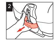
To fully recline, pull out on handle and push top of child restraint back.
